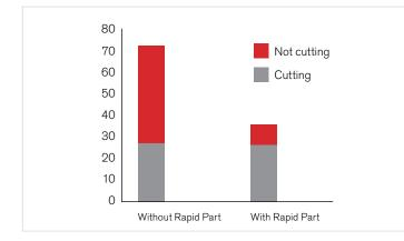
In this example, non-cutting time (red) is reduced by 80%, lowering the overall production time by 50%.
