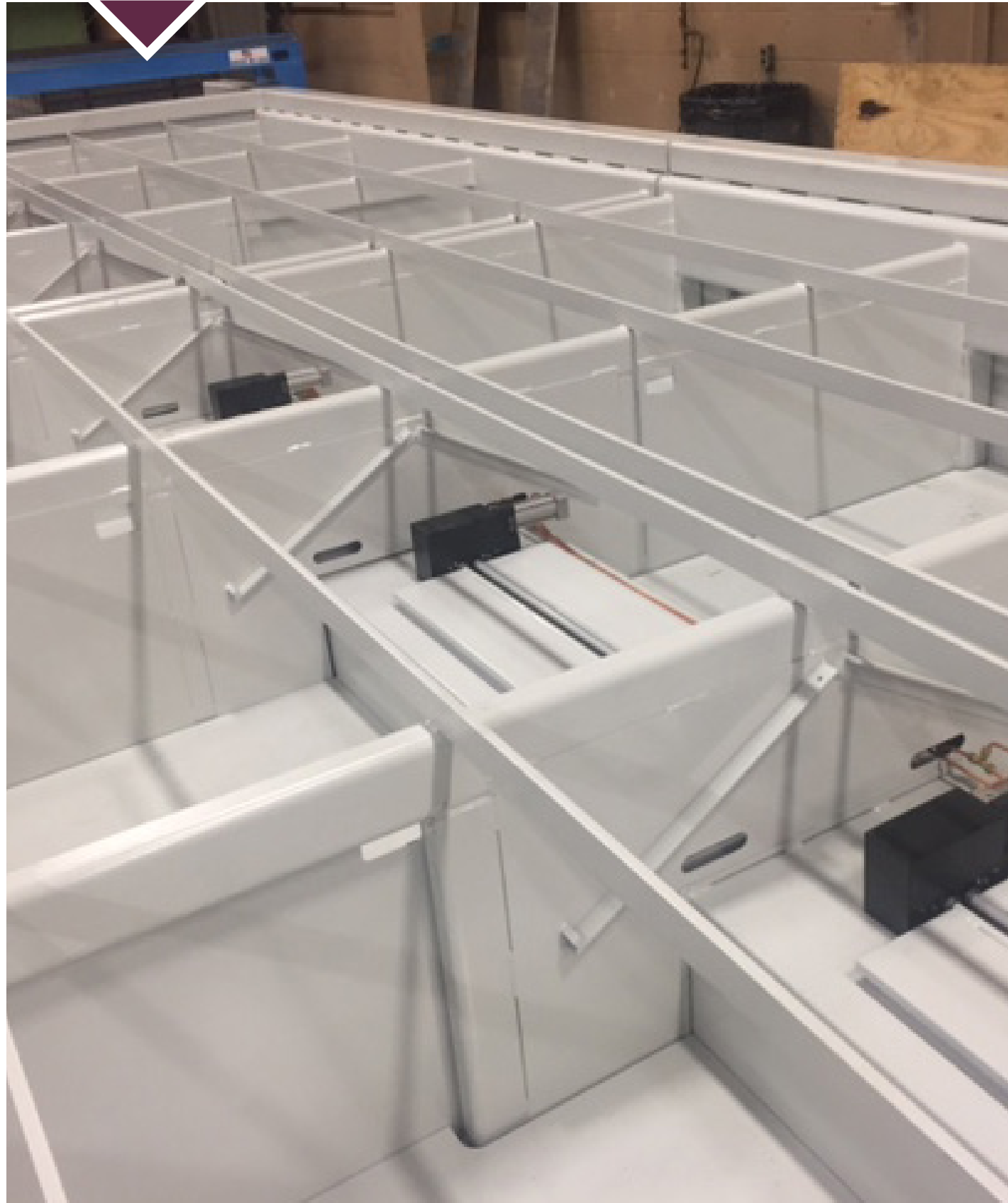
Figure 3. To efficiently handle high airflow, the space under the cutting surface of most industrial cutting tables is separated into zones down the length of the table.
