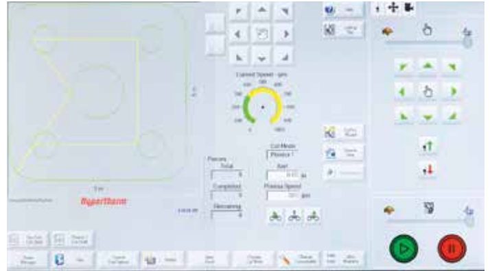
Phoenix software interface with Soft OpCon motion tab (at right), one of three out of the box consoles available.
